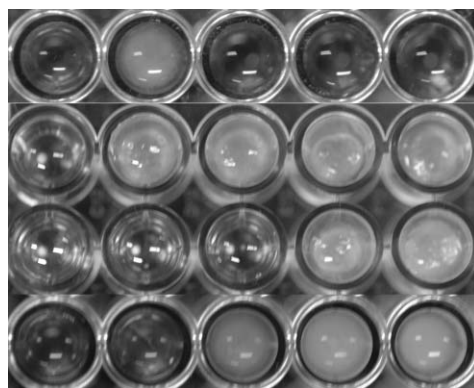
Fig. 4 Results of activities of three inhibitors: row 1) Left to right: sol. of 1 ; sol. of 1 and enzyme; sol. of 1 + 3 ; sol. of 1 + 4 ; and sol. of 1 + 5 ( [\mathbf{3}] = [\mathbf{4}] = [\mathbf{5}] = 33 mM); row 2) pamidronate; row 3) Zn 2+ ; and row 4) Na 3 VO 4 . (Left to right, conc. = 33; 3.3; 0.33; 0.033; 0.0033 mM).
